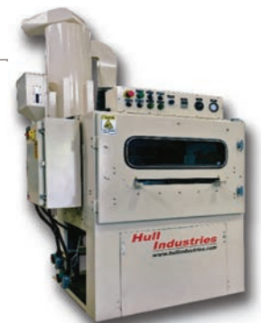
Workloading Frame Deflasher
